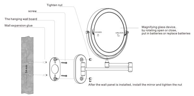
Use an impact drill with a diameter of 6mm and insert the expanded colloidal particles. Place the hanger plate on the hole and screw down
