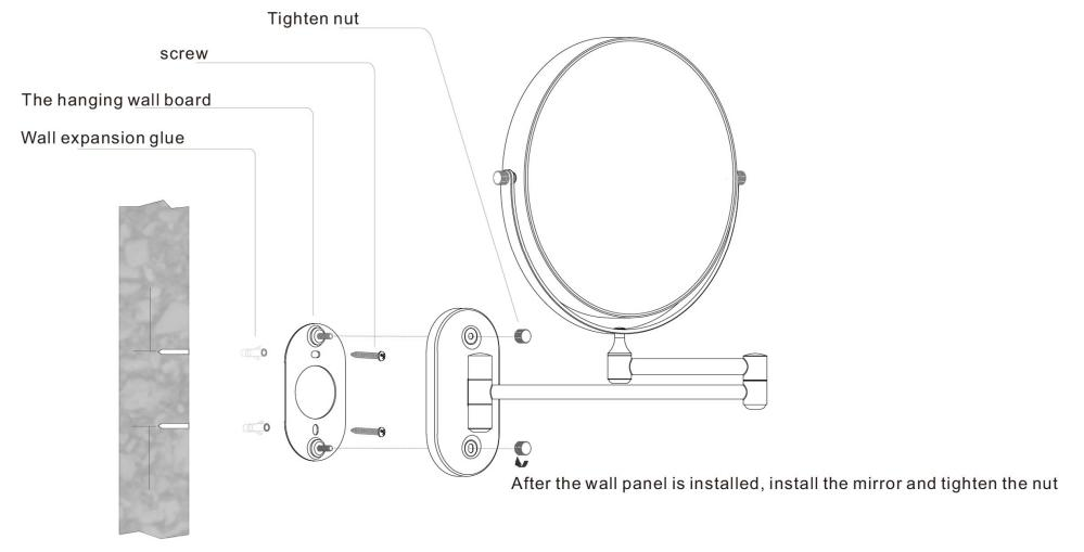
Use an impact drill with a diameter of 6mm and insert the expanded colloidal particles. Place the hanger plate on the hole and screw down
